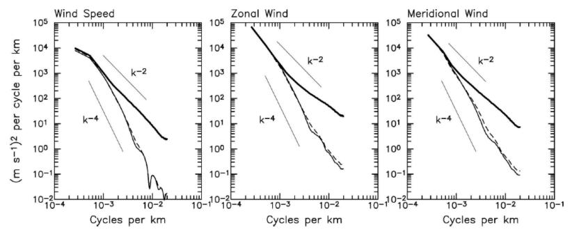
Along-track wavenumber spectra of (left) wind speed and the (middle) zonal and (right) meridional wind components in the eastern North Pacific for 2004 computed from QuikSCAT observations (heavy solid lines), NCEP analyses (thin solid lines), and ECMWF analyses (dashed lines) of 10 m winds bilinearly interpolated to the times and locations of the QuikSCAT observations. From *Chelton et al.* (2006).
