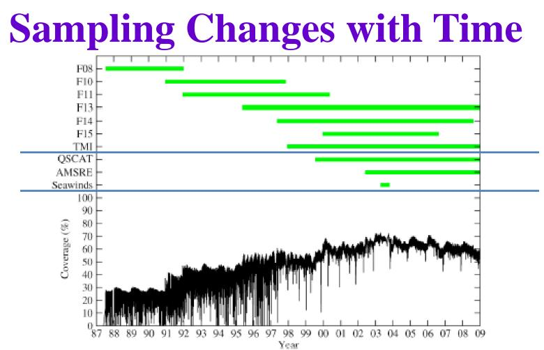
Time availability of satellite surface wind data sets. The SSMI/I instruments are denoted F08 through F15. The percentage of the global oceans observed by these missions in a 6-hour period is shown in the bottom portion of graph. From *Atlas et al. (2011)*.
