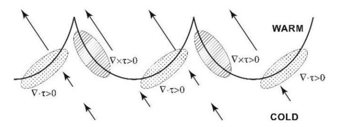
A schematic showing the observed SST influence on near-surface wind stress in regions of strong SST gradients. From *Chelton et al.* (2005).
